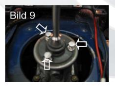
Now fasten the plastic ring using a cable tie onto the rubber seal. Screw the seal back on (see picture 13).
