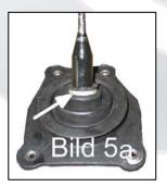
Now the plastic bearing holder on the small ball is forced away and installed onto the short shifter.
