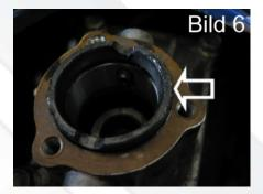
Lay the paper gasket on the seal surface and attach the distance flange. The pin needs to be adjusted so that it is above the original pin in the recess of the plastic bearing holder (see picture 7) Place the short shifter perpendicular to the transmission so that the pin slides into the bearing recess. Fasten the seal sleeve using the supplied screws. (see picture 9)
