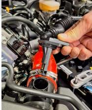
3.Loosen both clamps on the intake hose, pull the resonance hose out of the opening and put it aside. The intake hose can now be removed.
