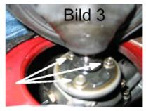
Note: only remove gear shifter whilst in neutral
