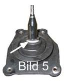
Now the plastic bearing holder on the small ball is forced away and installed onto the short shifter (1). The plastic bearing holder ring can now be prised off from the large ball using a small screwdriver in the plastic bearing recess of the gear stick. (see pictures 6 and 7)
