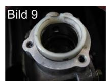
Lay the paper gasket (6) on the seal surface and attach the distance flange (5). The pin needs to be adjusted so that it is above the original pin in the recess of the plastic bearing holder (see picture 11) Now adjust the plastic bearing holder on the short shifter so that it lines up with the plastic bearing recess (see picture 12)
