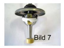
Lay the white plastic bearing holder (2) with washer on the short shifter ball and press on the new rubber seal (3) (see picture 7)
