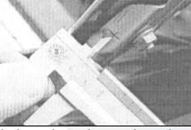
4) Using a 5mm drill bit, drill a hole at the point you have just marked on each hinge.
