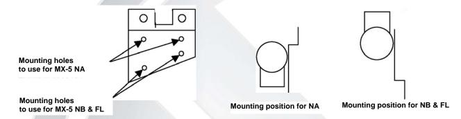
Unscrew the fixing nuts for the trunk key lock and mount the steel mounting plate and motor here. Hook the steel operating rod through the motor and shorten it to the required length.
