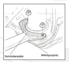
Place the brace bar loosley on to the top mount studs ans ensure it is all sitting level. Then refit the nuts and tighten down the bar.
