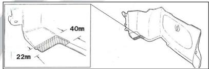
Left hand side cut out as shown, including the metal part.
