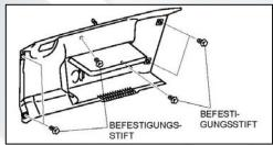
For the side trims. Remove all the fasteners as show below, and remove the two trims. For the metal trim remove all screws.
