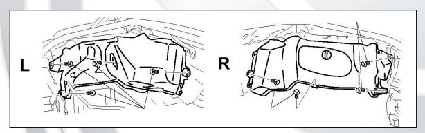
Undo the top mount retaining nuts as show below, and also the cable retainer nut.
