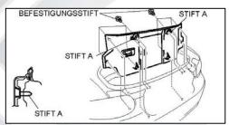
Remove the fasteners in the partition board, and then remove the trim.
