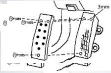
Hold the pedal plate to the accelerator pedal and mark the mounting holes. With a 4 - 4,5 mm drill bit, drill holes on the marked positions. Install the plate with the supplied fittings.
