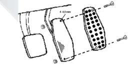
The clutch and brake pedal cover are installed as follows. Slide the cover on to the bottom part of the pedal plate. Now use a small screwdriver to pry the rubber on to the top part of pedal plate
